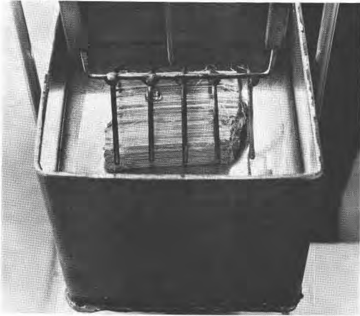
FIG. 2. Close up of mercury container (Fig. 1) showing relationship of pointer, sample holder, and mercury. Dimensions of mercury container are 4\frac{1}{2}'' \times 5'' \times 4\frac{3}{4}'' .
