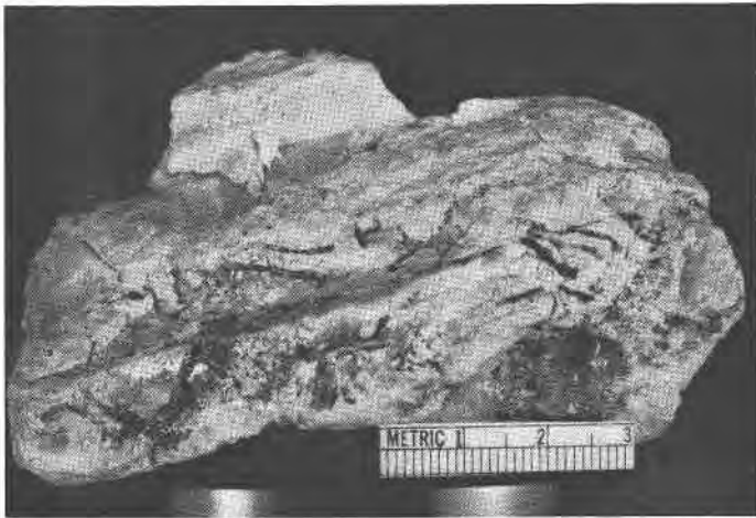
FIG. 3. Back of piece shown in Fig. 2 showing borings lined with manganiferous material. One large boring appears above 2.4 on the scale. Each small division of scale is 1 mm.
