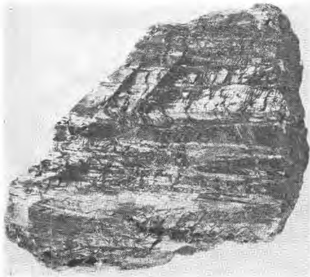
FIG. 4. Kinking in a deformed single crystal from the Zeehan fault zone, Tasmania; \times 1\frac{1}{2} .
