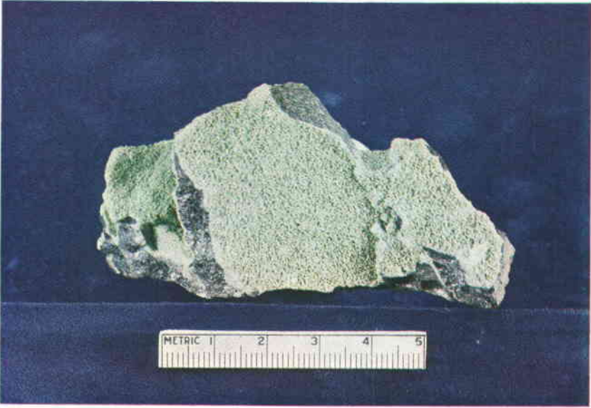
FIG. 4. Nickel-gymnite of Genth (1851), later called genthite by Dana (1867), coating chromite from the Wood's chrome mine near Texas, Little Britain Township, Lancaster County, Pennsylvania. U.S. National Museum No. 82525.
