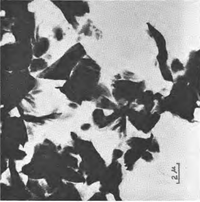
FIG. 2. Electron Micrograph of the 2\mu to 1\mu equivalent spherical diameter fraction of the Bayard, New Mexico montmorillonite.
