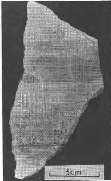
FIG. 6b. Alternating beds of predazzite (mottled) and dolomitic marble. Specimen M4. Chemical and petrographic data for this specimen are given in Table 2.
