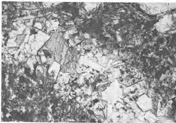
FIG. 11. Extreme residual fraction consisting of alkali feldspar, quartz and calcite, as a veinlet cutting modified hawaiite (Re 32), in upper part of sill; uncrossed polars, \times 23 .
