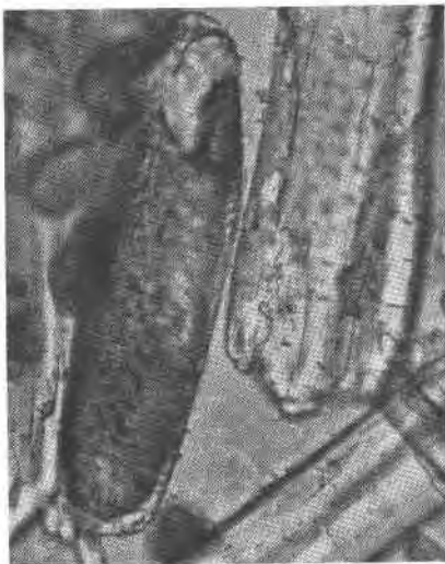
FIG. 3. Photomicrograph of a dark rind of anhydrite (?) on a prismatic grain of gypsum (colorless). Note incipient development of rind material in cleavage crack of large, colorless (recrystallized) gypsum plate. Data: Run LS 51, gypsum stirred in 22% \text{H}_2\text{SO}_4 solution at 50°C and 1 atm for 211 days. About 50% conversion to anhydrite at end of run. No reaction was observed until 146 days. Magnification about 250X.
