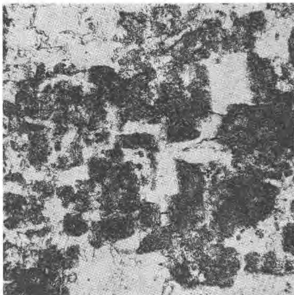
FIG. 3. ( \times 96 ) Rhodochrosite (dark grains) partly replaced by magnesian kutnahorite (pale grains). Polarizer only. Ryûjima mine.
