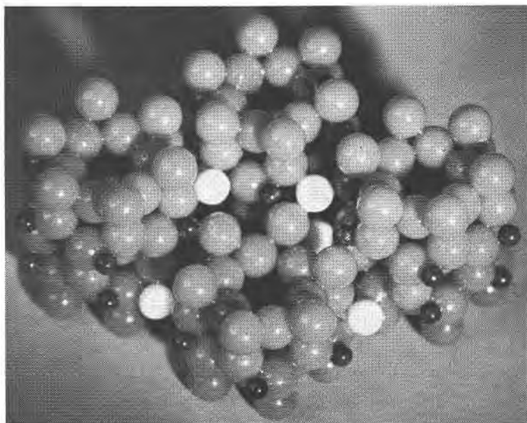
FIG. 8. Model of the crystal structure of beryl. Stacking of hexagonal Si_6O_{18} rings is shown. Oxygen ions are represented by the grey balls. White balls show aluminum ions in octahedral sites. Small dark balls are the Be^{++} ions in tetrahedral sites. Channels formed by the hexagonal rings are evident.
