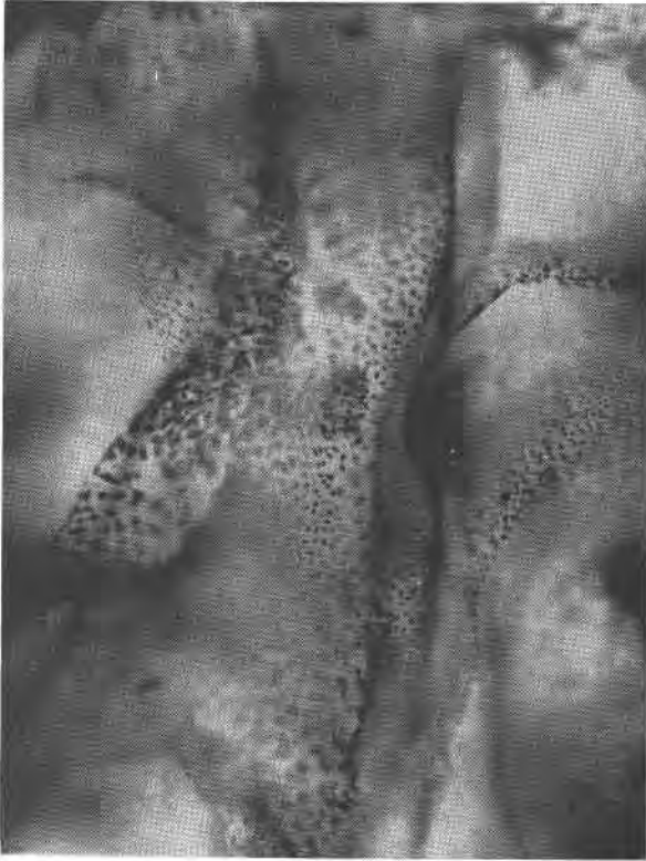
FIG. 4. Photomicrograph of wisp- or veil-like inclusions in V_2O_5 flux-grown emerald. Basal section, 150X.
