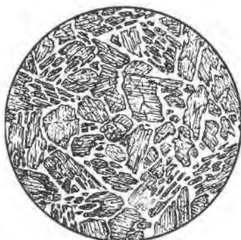
FIG. 1. Typical texture of jadeite from Manzanal, Guatemala. Jadeite grains, many of which are small fragments with uniform crystallographic orientation, are surrounded by clear, untwinned albite. Some jadeite grains have very thin rims of analcite. Diameter represented by drawing about three millimeters.
