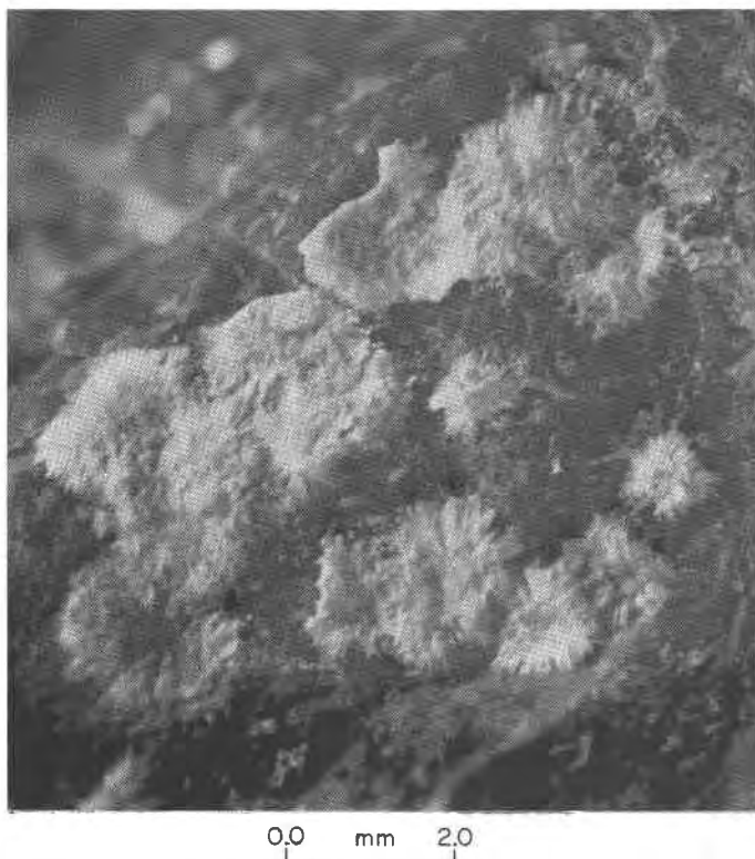
FIG. 2. Photograph of hand sample showing flattened rosettes of white, silky rhodesite on silicic volcanic rock.
