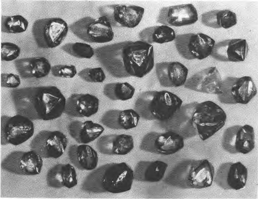
FIG. 1. Diamonds recovered during gold mining operations. They are all colored consistent with having been irradiated by high energy alpha or beta particles.
