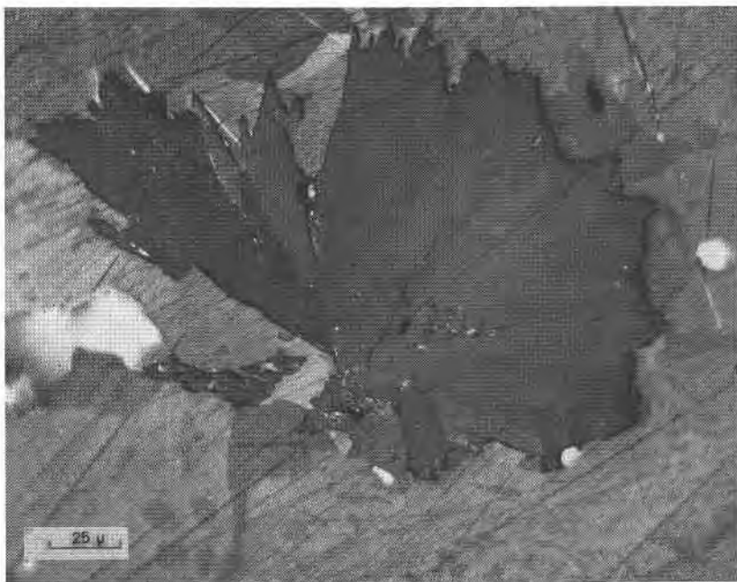
FIG. 3. Photomicrograph of radial aggregate of antimonian loellingite, medium and dark gray, in paradocrasite containing blebs of stibarsen. Nicols partly crossed.
