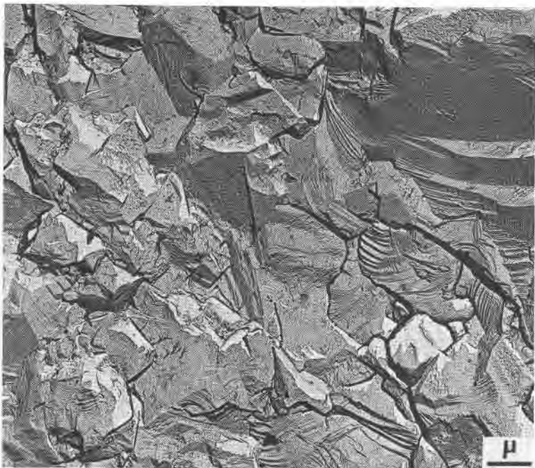
FIG. 6. Electron micrograph of fracture interface of Ubangi carbon, showing both intergranular and transgranular fracture. (Replica)
