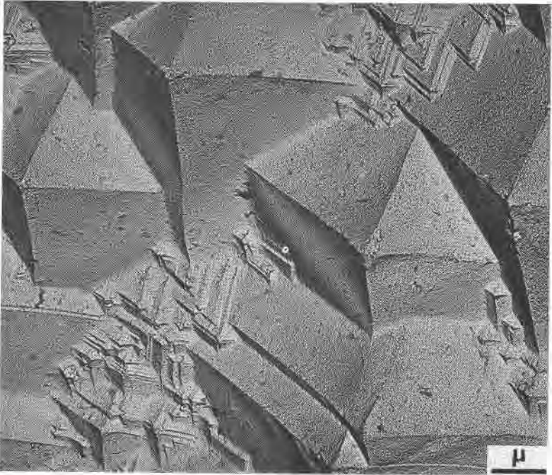
FIG. 8. Fracture interface of 250 \mu\text{m} diamond crystal embedded in the polycrystalline matrix. (Replica)
