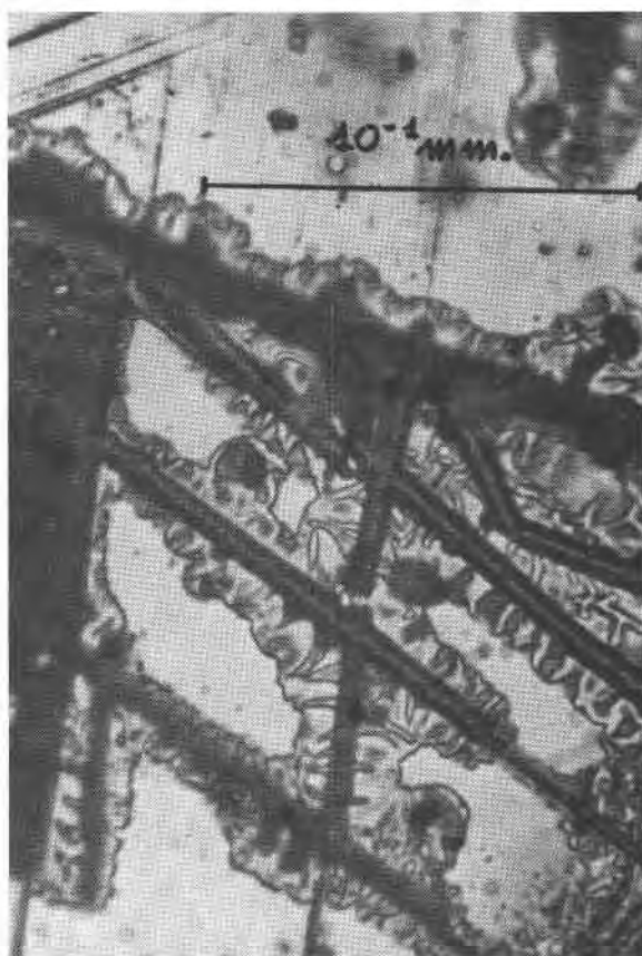
FIG. 2. Filling process of the goethite framework.
