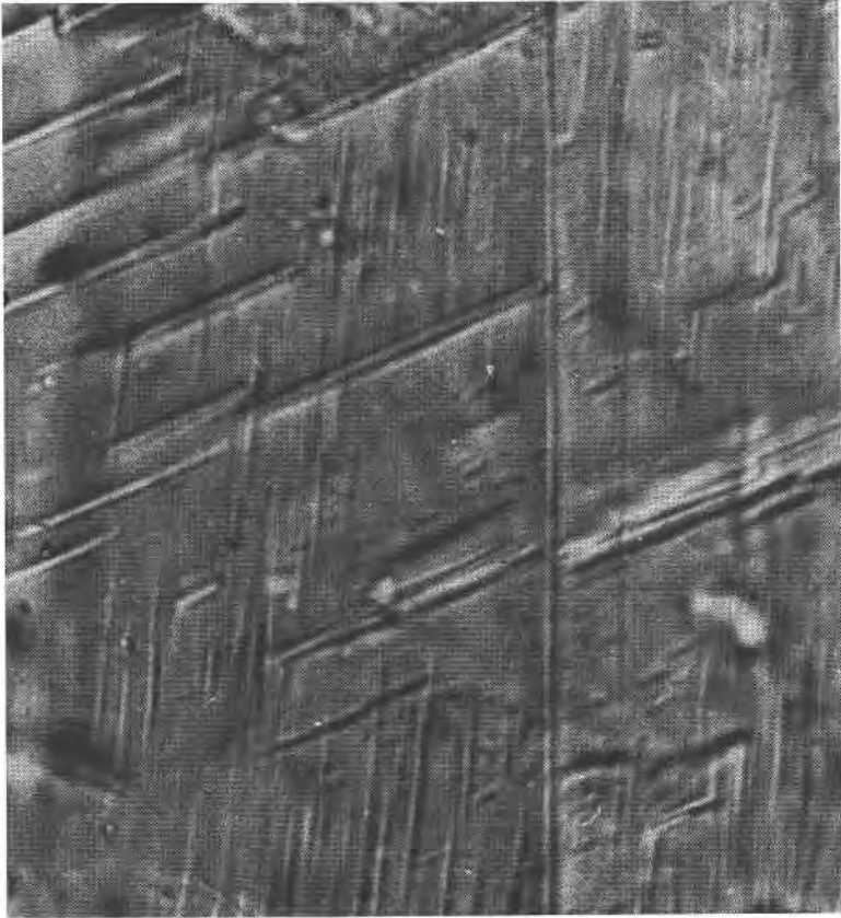
FIG. 1. Photomicrograph of augite from pyroxene granulite, Hudson Highlands, New York (Jaffe and Jaffe, 1971). View normal to (010) showing three sets of exsolution lamellae (set text and Table 5). One set represented by the prominent continuous lamella (vertical) is oriented parallel to (100) of the host. A second set of fairly coarse lamellae lies at a 116^\circ angle to the c -crystallographic axis. A third set of very fine lamellae lies in the acute angle \beta at 6^\circ to the c -crystallographic axis. The coarsest lamellae are 1.0 \mu\text{m} thick.
