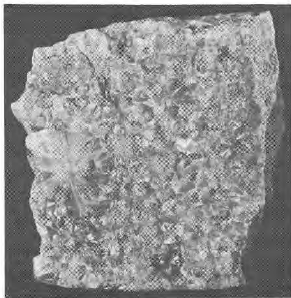
FIG. 5. Dawsonite infilling a joint in a quartz lithic sandstone from the Singleton Coal Measures. The specimen measures 1\frac{3}{4} inches across.
