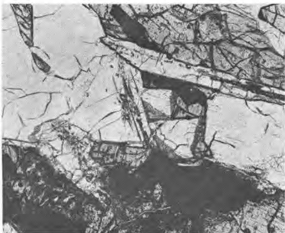
FIG. 1. Tridymite crystal, 1.5 \times 0.1 mm, associated with anorthite (white) and augite (gray), in lunar rock 15085 (Smithsonian Institution photograph).
