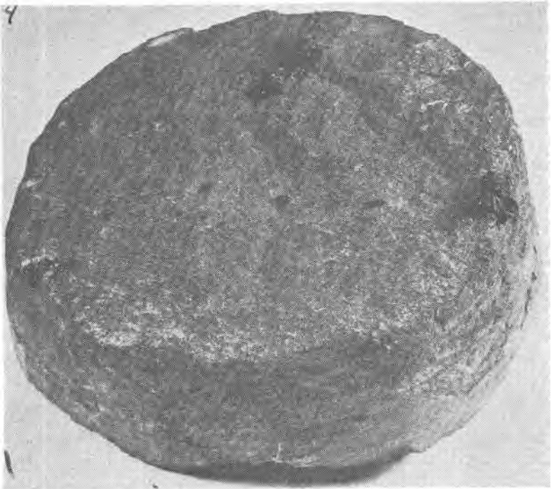
FIG. 4. Section of 4-inch drill core from O. L. Johnson #1 well, 4853 ft, Uinta Basin, Utah, showing large crystals of leucosphenite in dolomitic marlstone.
