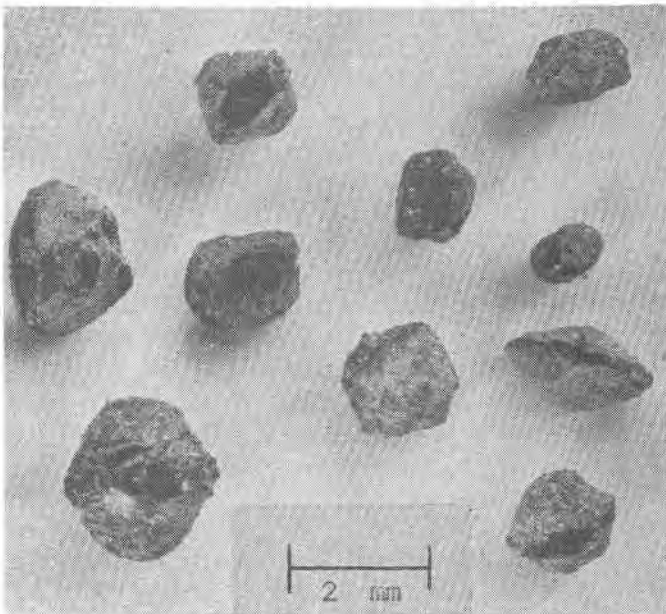
FIG. 1. Leucosphenite, Kermit Poulson well #1, 4500-4510 ft. Discoidal crystals heavily impregnated with brown shale matrix. Only an equatorial zone of prism faces is developed.
