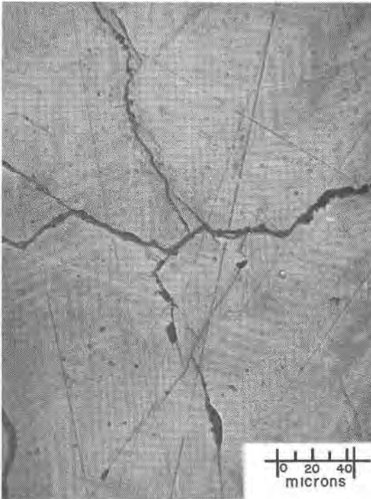
FIG. 3. Photomicrograph showing details of twinning in haycockite.
