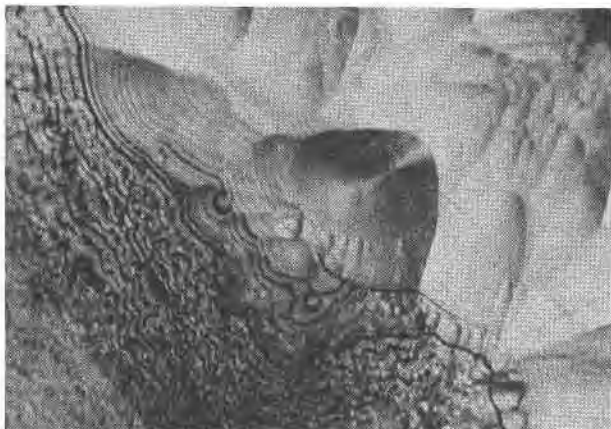
FIG. 2. Fine-layered hetaerolite encrusted with a weakly recrystallized zone of the same mineral. Polished section, oil immersion, magnification 930 \times . (a) parallel nicols (b) crossed nicols.
