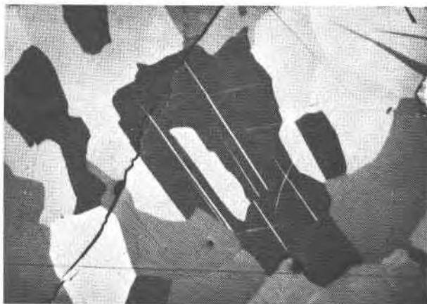
FIG. 3. Grained balkanite with polysynthetic twins. Crossed nicols. Magnification 330 \times .
