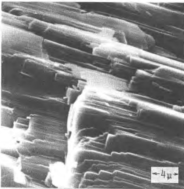
FIG. 2. Scanning electron micrographs of the fracture surfaces of jadeite. Note the extensive transgranular cleavage characteristics of the crack propagation.
