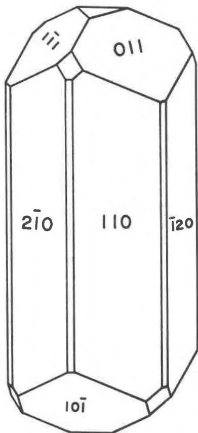
FIG. 1. Axonometric projection of an idealized crystal of yedlinite. The c axis is vertical, and a_2 is to the right. Faces of the two most important forms are indexed with the superfluous i index omitted.
