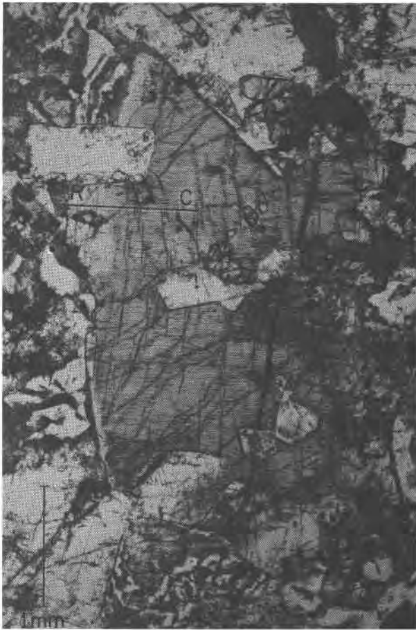
FIG. 2. Photomicrograph of augite grain enclosing plagioclase and orthopyroxene optically showing light rim developed against quartz-perthite intergrowth in specimen U.568 (Hewins, 1971, p. 122). CR is traverse line from core to rim shown in Figure 3.
