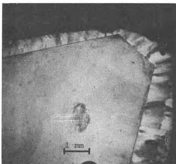
FIG. 1. Photomicrograph of zoned Li-mica crystal revealing a central muscovite core bounded by \{110\} and \{010\} faces surrounded by an external rim composed of lepidolite crystallites. Note the absence of irregularities and embayments on the muscovite faces. The blemish near the center of the muscovite is an abrasion on the cleavage surface.
