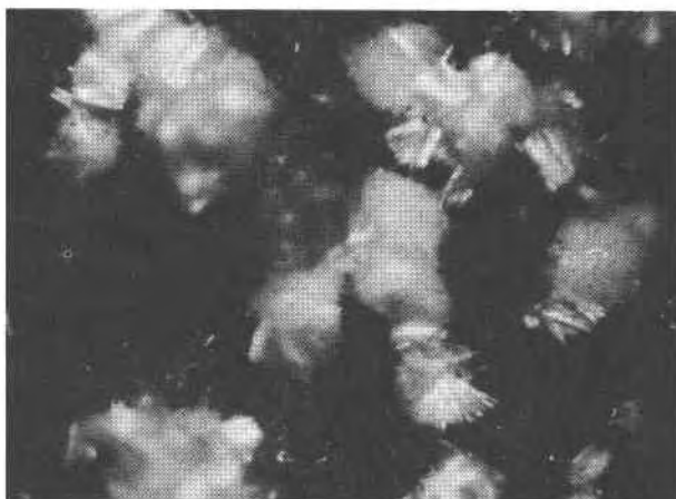
FIG. 1. Studtite forming aggregates of needle-like crystals on limonite, Menzenschwand, Southern Black Forest. Magnification about 60 X.
