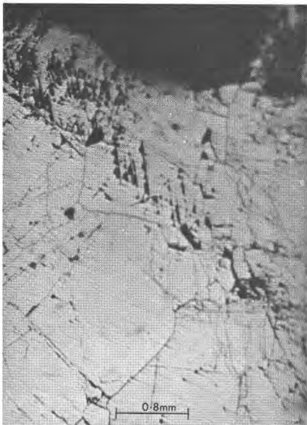
FIG. 3. Triangular pits (or facets as in Fig. 6) in rhombic and triangular zones limited by cleavage planes. Two magnifications of the same area show the patterns.
