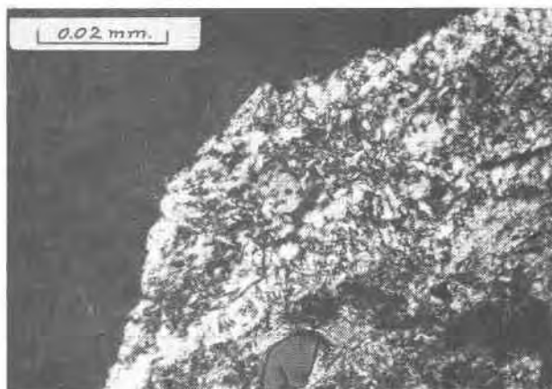
FIG. 2. Detail from Figure 1. The crust is seen to consist of somewhat oriented clay particles, with optical characteristics resembling those of smectite. Transition from the crust to the mass of the ped appears sharp.
