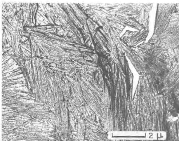
FIG. 4. Electron transmission photograph of a replica prepared from an undisturbed palygorskite crust. The palygorskite fibers are arranged in the form of thick mats, subdivided into approximately parallel strips. Within each strip the fibers have again a more or less parallel orientation.
