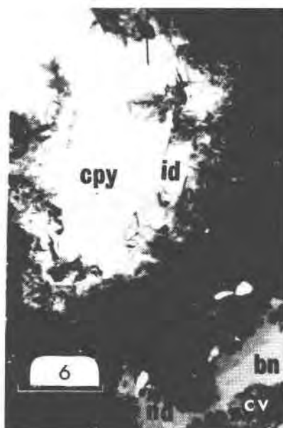
FIG. 6. Chalcopyrite (cpy) replaced by idaite (id) in turn replaced by covellite (cv). At bottom right bornite (bn), replaced by digenite (nd) in turn replaced by covellite (cv). Scale bar = 400 microns.
