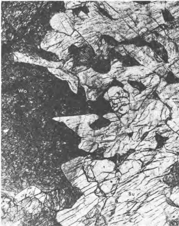
FIG. 1. Photomicrograph of coexisting wollastonite (turbid) and bustamite (clear) in a specimen from Franklin, New Jersey (width of field is 8 mm).
