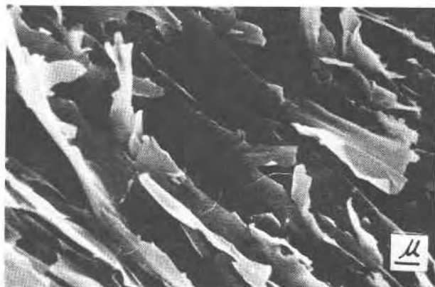
FIG. 4. Scanning electron photomicrograph of swinefordite.
