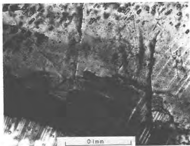
FIG. 3. Small bulge, which may be a potential grain nucleus, in an irregular (migrated) deformation band boundary. Note the general paucity of inclusions in the area of movement of deformation band boundaries. Crossed polars.
