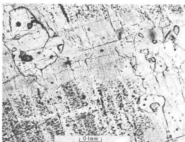
FIG. 5. Recrystallized grains and aggregates of plagioclase (clear of minute inclusions) generally surrounded by a zone of host grain containing minute inclusions, surrounded in turn by unaffected plagioclase containing larger inclusions. The apatite occurring as grains and inclusions in the recrystallized plagioclase aggregates is much coarser-grained than the inclusions in the surrounding plagioclase. Plane-polarized light.
