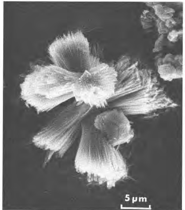
FIG. 10. Platy and spindle-fiber type ferrierite crystals. X-ray microprobe analysis reveals that both types are essentially pure K-ferrierite. The crystals in the upper right are pure silica-quartz crystals with ferrierite in this metastability region. Starting composition: 1.63NaO-1.63K_2O-Al_2O_3-13.5SiO_2-130.4H_2O-0.88CO_2-2.44(HCO_2)_2 , 230°C, 92 hours.
