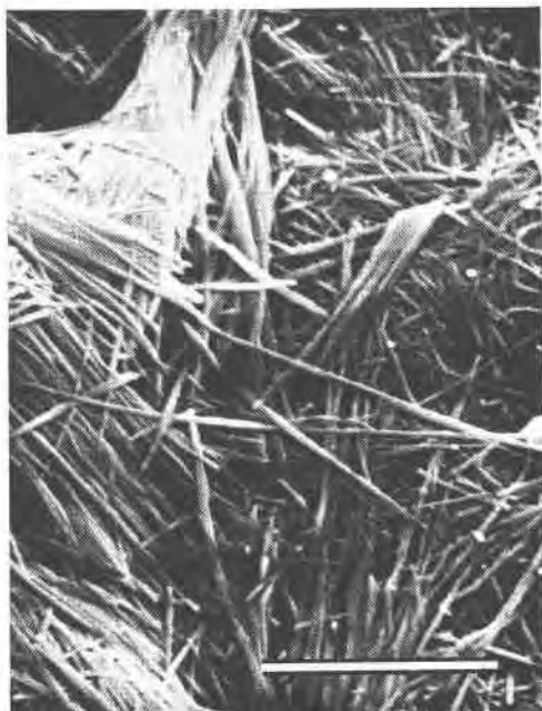
FIG. 4. Detail from Figure 3 showing palygorskite fibers at the junction of two strips. The strips generally consist of longer fibers (often > 3\mu ) becoming interwoven at the strip junctions, see top left of figure. Areas between the strips are occupied by poorly aligned smaller fibers (often < 1\mu in length). Bar is 2\mu long.
