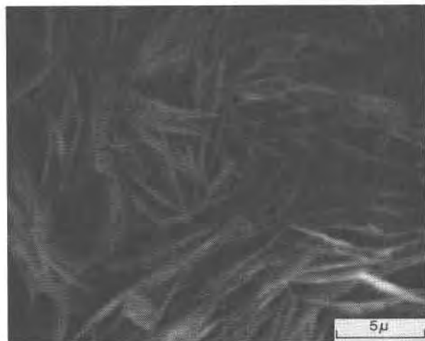
FIG. 2. Part of a carrboydite nodule, at higher magnification, showing the platy nature of the crystallites.
