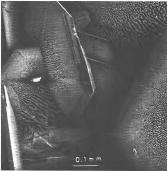
FIG. 5. Scanning electron micrograph of offretite overgrowths on levyne from Queen Creek, near Superior, Arizona. Note that the offretite fibers have grown only on the basal faces of the levyne.
