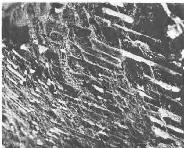
Fig. 1. White rodding in the kaersutite xenocryst; note the slight change in direction of the rodding and the smooth furrows where the rods have been removed. Photograph is 7 cm wide.
