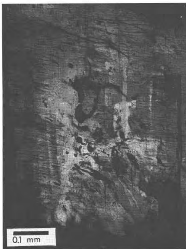
FIG. 1. Feldspar crystal with skeletal plagioclase core (light gray) and sanidine mantle (dark gray); overgrowth has fine lamellar plagioclase-sanidine intergrowth, Capsule 351.
