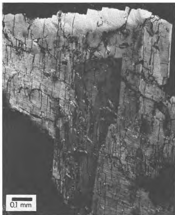
FIG. 3. Feldspar crystal with sharply defined zones that reflect the step-cooled history (see text for details): (a) photomicrograph; (b) sketch delineating the zones. Capsule 510.
