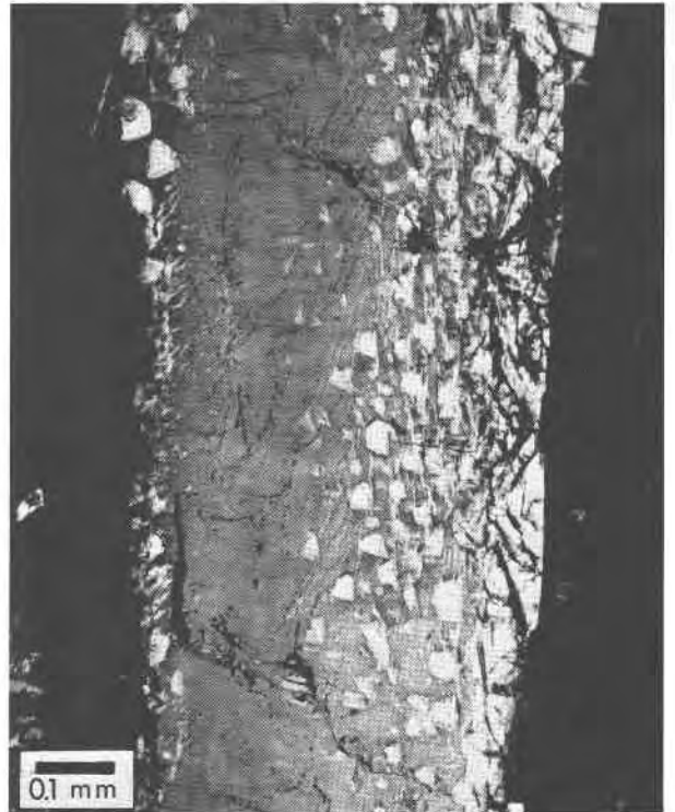
FIG. 5. Sanidine crystal with patch-plagioclase intergrowths; the patches on each side have a common extinction angle. Capsule 514.
