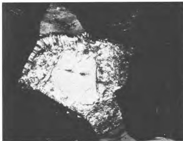
Fig. 2. Crossed-polarizer micrograph of a coesite grain about one mm across in sample SRV-1, showing radial growth of quartz from rim toward center.
