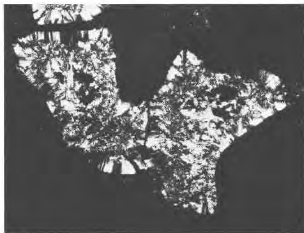
Fig. 3 and 4. Crossed-polarizer micrographs of polycrystalline aggregates of quartz in sample SRV-6, showing the characteristic radial growth texture around the rim. All of the coesite in this specimen has inverted to quartz. The approximate dimension across Figure 3 is 8 mm and Figure 4 is 5 mm.
