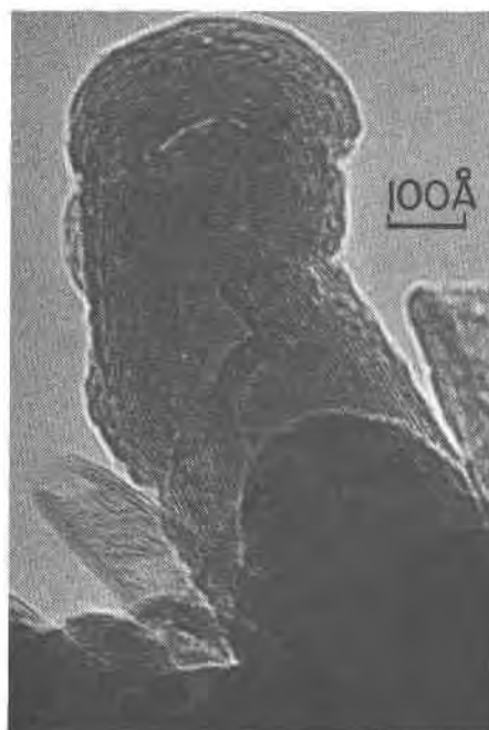
Fig. 10 Microstructure of a fibril showing bump-like growth (Run OS 144).
