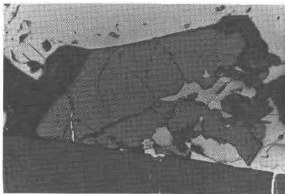
Fig. 1. A somewhat irregular manganochromite grain (pale grey) lying between hexagonal pyrrhotite (white) and a large diopside crystal (grey). Width of field 450 \mu m.
