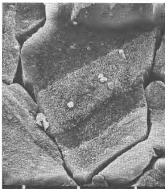
Fig. 6. Two views of the same part of a natural surface on a ulexite fiber bundle, taken with a Cambridge 180 scanning electron microscope by R. L. Oscarson, U.S. Geological Survey. Distance between scale marks is 3 micrometers: (a) magnification 990 \times (b) magnification 2590 \times .
