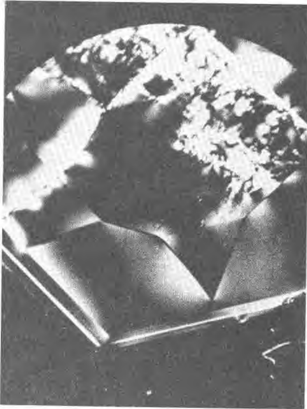
Fig. 9. The polygonal structure in a section cut perpendicular to the c axis of a beryl crystal (from Sahama, 1966, pl. II, d).
