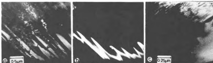
Fig. 4. Electron micrographs of exsolution textures. (a) (100) exsolution of two ordered phases (both with antiphase domains); dark-field, g = 101 , 97667. (b) Same area as (a); dark-field, g = 202 . (c) Patchy exsolution of omphacite in impure jadeite, approximately parallel to (010); bright-field, 119428.
