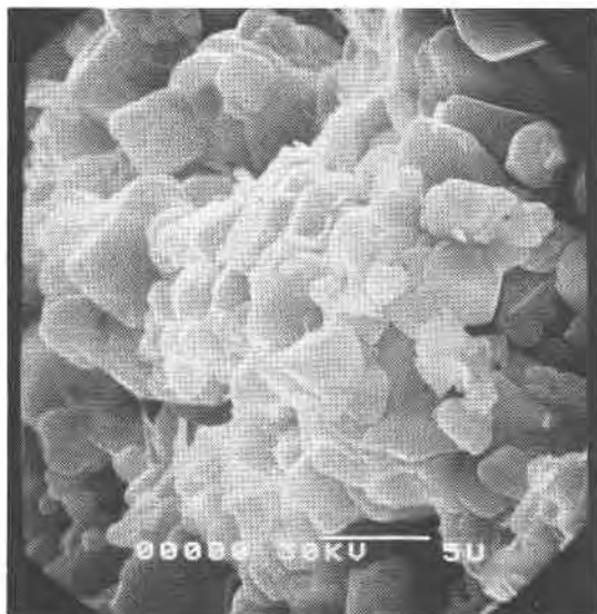
Fig. 3. Scanning electron micrograph of synthetic Cs-dioctahedral mica. Bar is 5 microns.
