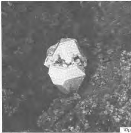
Fig. 4. BE image of bromian chlorargyrite crystal [Ag(Cl,Br)] in goethite; broken surface; uncoated, 30kV. Heavy trace elements are easily found, even on a fracture surface, if concentrated in such specific phases.
