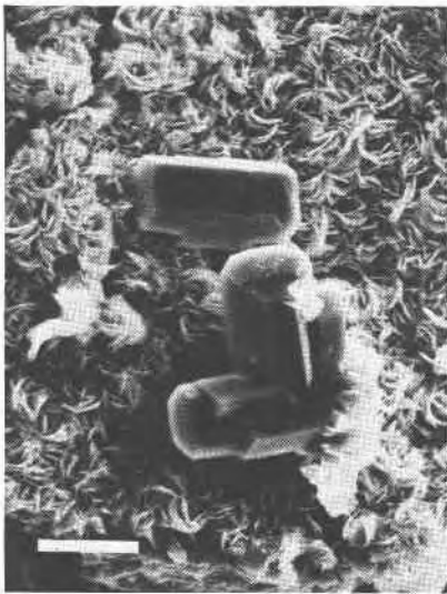
Fig. 1. Scanning electron photomicrograph of mitridatite (feathery crystals) and associated hydroxy-apatite (hexagonal prisms). The white bar in the lower left corner represents 10 \mu\text{m} .
