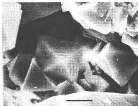
Fig. 1. Scanning electron photomicrograph of hydrated aluminum hydroxy fluoride octahedra, Sobu A, from Big Southern Butte, Snake River Plain, Idaho. Bar scale is 10 microns. (Photo by James Nishi, U.S.G.S.)
